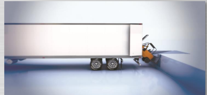
Trailer separation from Loading Dock
