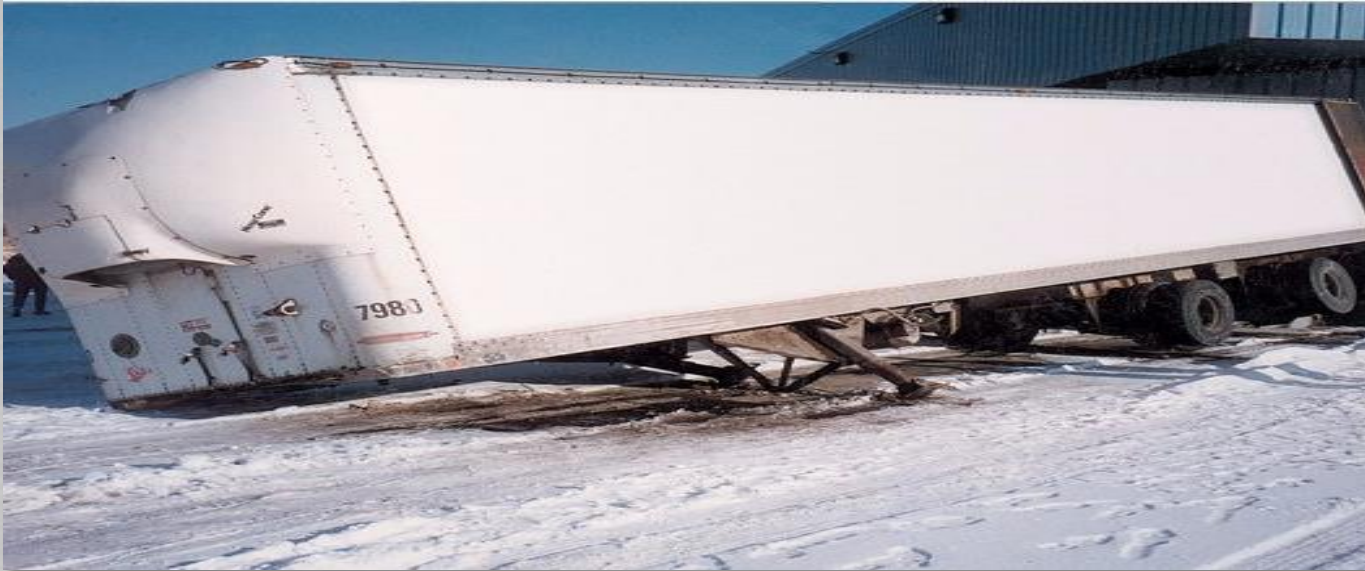
Landing Gear Collapse
