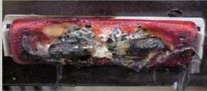
COMPRESSED INTO FOAM SEAL, LIGHTS CAN REACH 900 DEGREES F IN AS LITTLE AS 20-30 MINUTES.
