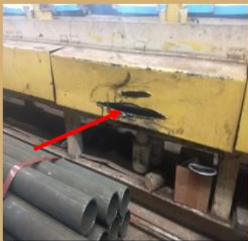
A guard that is damaged
