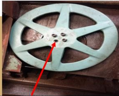
Flying wheel that is missing a bolt
