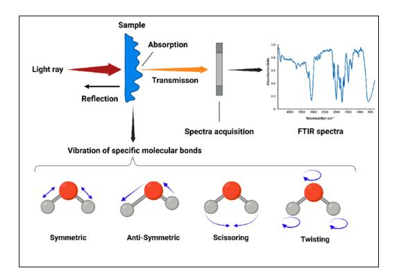
https://www.researchgate.net/figure/nfraredspectroscopy-measures-the-interaction-of-infraredradiation-with-matter-Upon fig1 381354000 When **Infra-red (IR)** radiation is passed through an air sample, some radiation is absorbed
