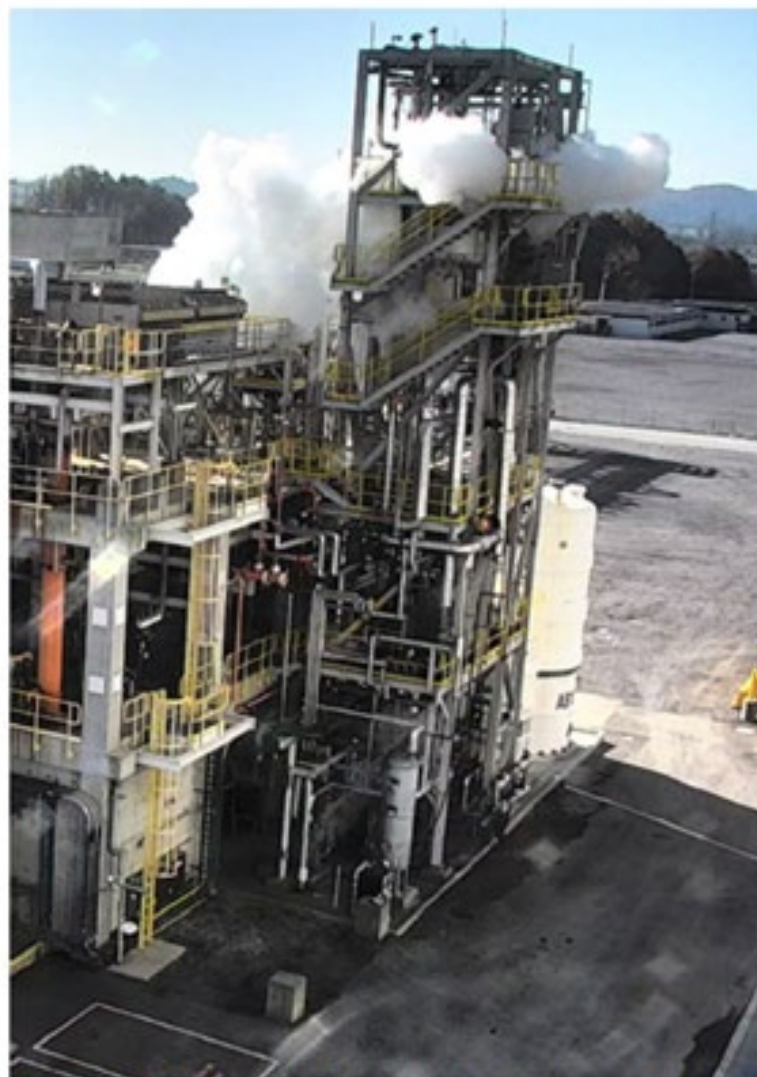
Figure 10. Image of HCl release at the time of release (left) and 15 seconds after release (right). (Credit: Wacker)
